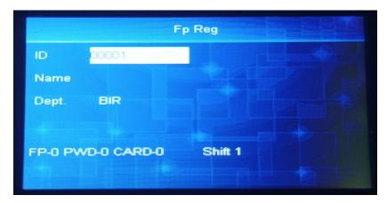
6. Once the biometric ID has been finished, hit the arrow right to access the name field, and then OK. Input the user's name, "Ex.JHON" (using the arrow keys to input a value or letters in upper and lowercase).
